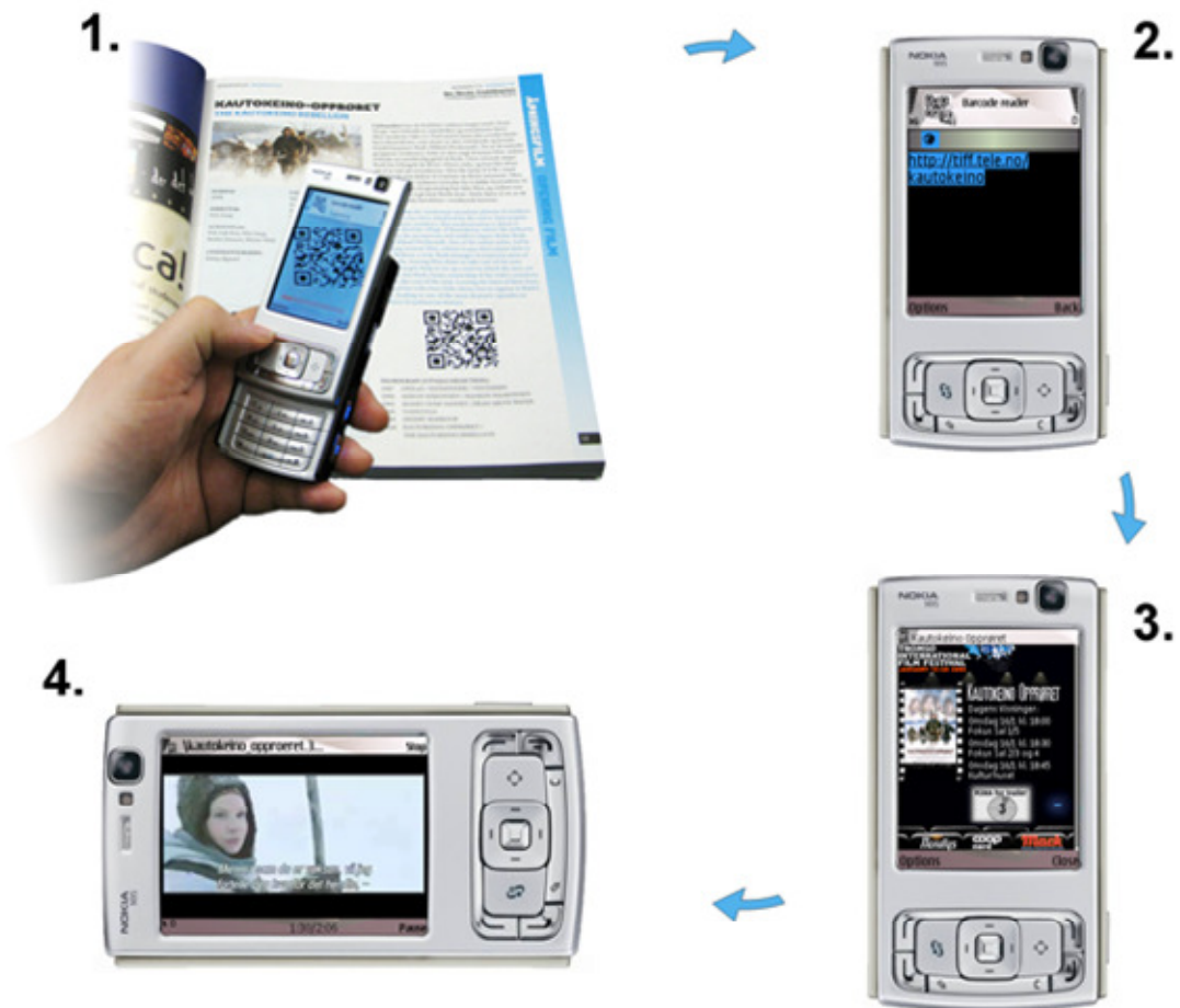
Figure 2.2 Interaction steps in the TIFF prototype.
