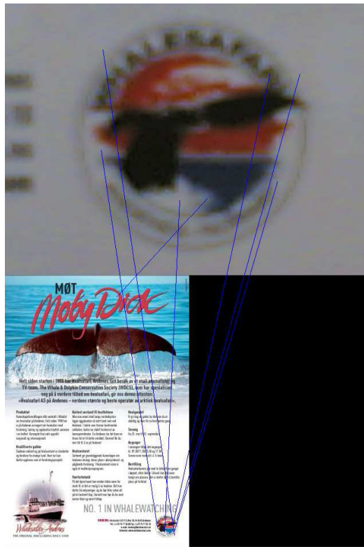
Figure 18: Best match illustrated for Mobil_MobyDick_merke.jpg. SIFT has correctly identified the source image to be part of the MobyDick advertisement.
