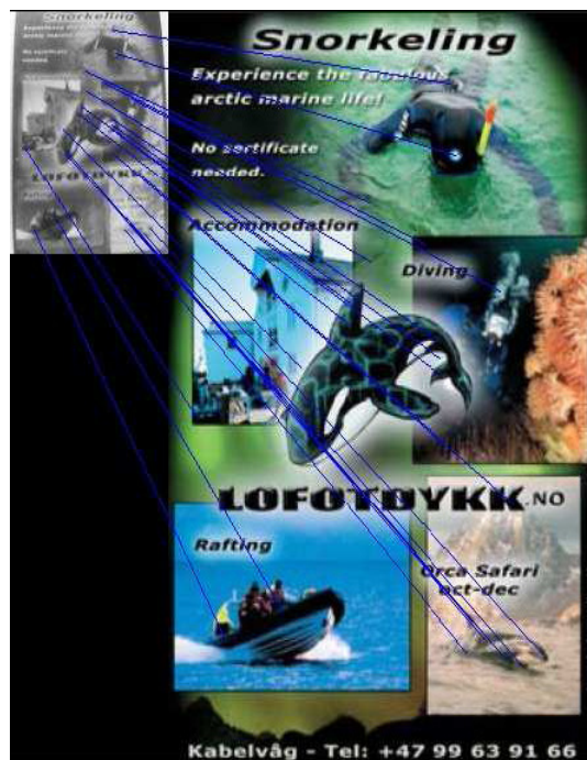
Figure 21: We have removed the colour from the search image, but the keypoint descriptors generated by SIFT are not affected. The match is correct.
